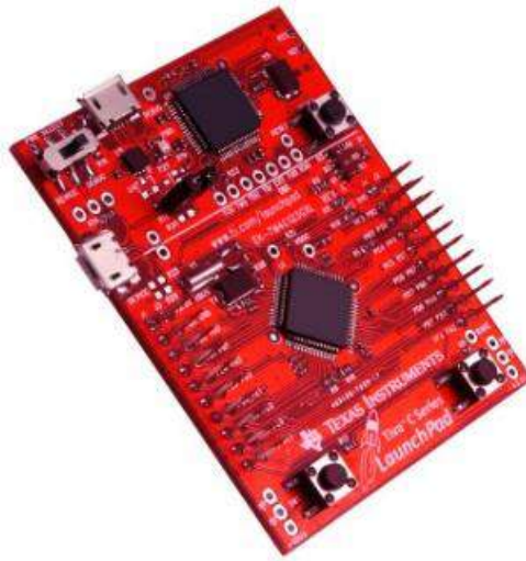
Figura 26 - TIVA™ C Series TM4C123G Launchpad
