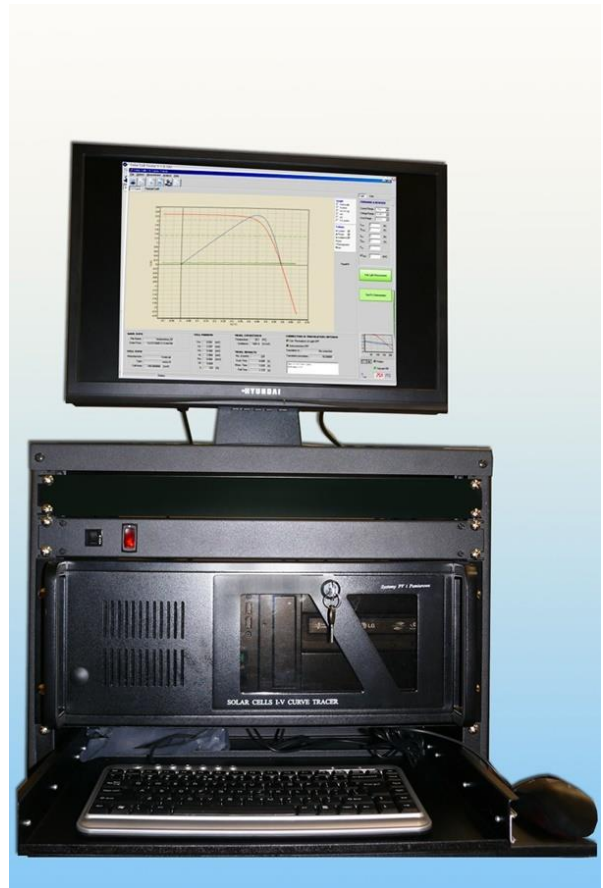
Figure 3: Typical I-V System Console – 15A/20A Current
