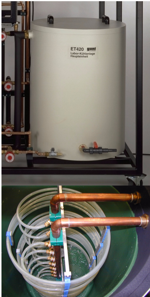
Fig. 3.12 Insulated ice storage (top) Interior view of ice storage (below)
