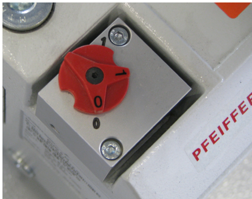
Fig. 3.9 Closed gas ballast valve
